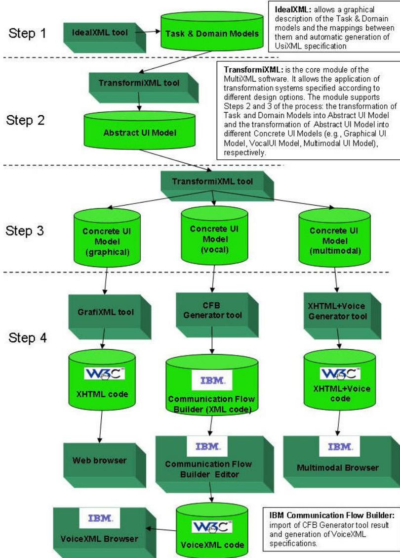
Figure 10. MultiXML software modules.
