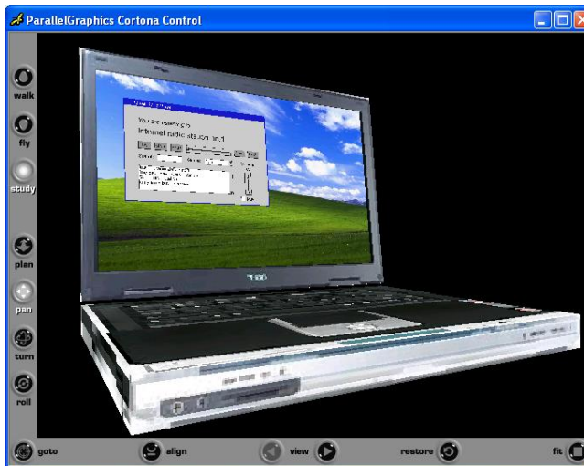
Figure 11. The virtual laptop with the GUI rendered in VRML97.
