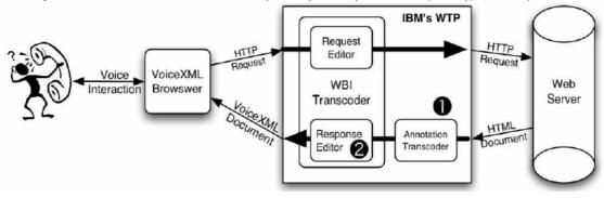
Figure 3-30 The VoiceXML Transcoder Architecture
